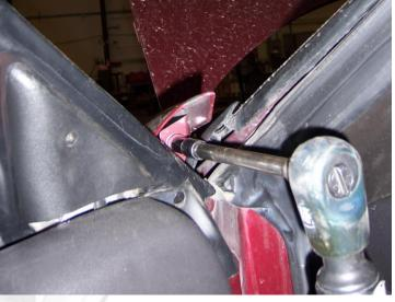
Remove the mounting bolts along the upper edge of the fender and carefully remove the fender.
