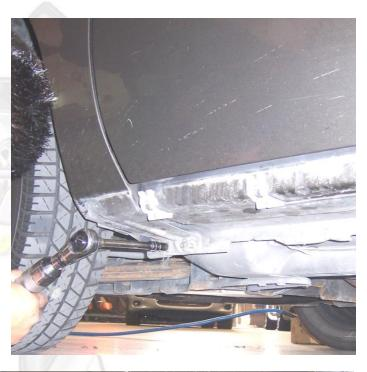
Open the door and remove (1) 10mm bolt located between the windshield pillar and the factory door hinges.
