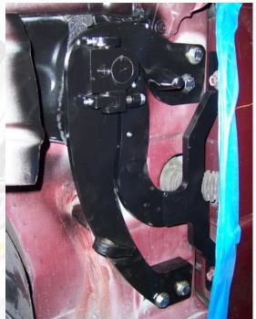
Hint\* Tighten the bolts on the door first then the bolts on the apron.
