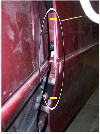
14) Close the door and Replace the fender, by reversing step 2 and 3.
